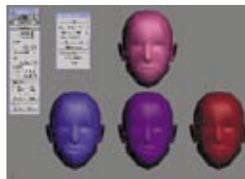
● New symmetry tools translate vertex offsets between objects: the purple head is the pink head plus opposite halves of the other two
